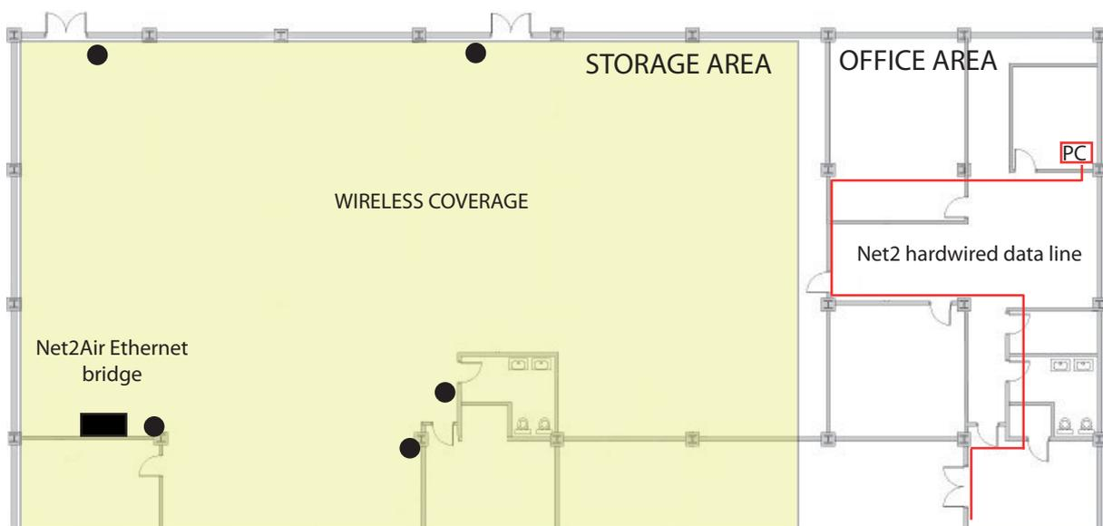
Fig 3. In this example we have an open storage area and a more complex office environment. We would recommend using wired Net2 ACU's for the offices and wireless ACU's with a Net2Air Ethernet bridge to cover the storage area, removing the need for long cable runs. This uses the benefits of each system.
