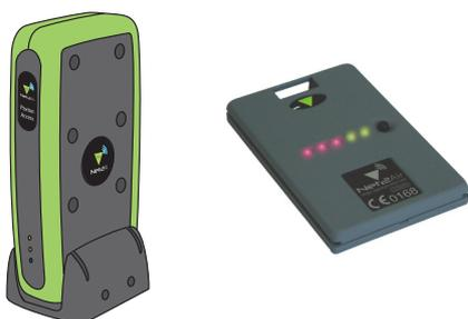
Providing all LED's light up, it is a suitable location to install the equipment. If not, a new location should be found and checked until all the LED's are lit. Try re-locating the wireless controller or bridge into a more direct 'line of sight'.
